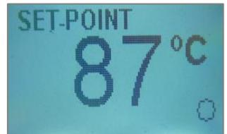
If neither key is pressed for approximately 5 seconds, the TC will return to the main screen and display the current process temperature.
