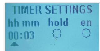
With the arrow positioned under the "hh" box the hour value can be set using the  $\Delta$  or  $\nabla$  keys.
