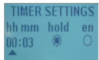
With "Hold" enabled the timer will not start until the temperature set point is reached. If "Hold" is disabled then the timer will begin as soon as the TC
