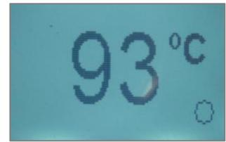
The box on the lower right of the screen is filled when heating is on.
